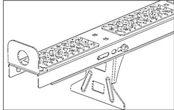
• Foot can be adjusted inward and outward, as well as angled, as slot allows.
