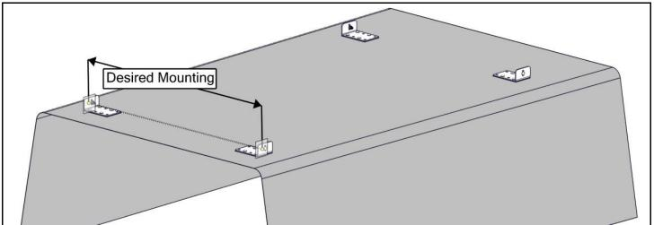
• At the width desired, find the corresponding slots on the ladder rack cross bow and attach mounting feet as shown.
