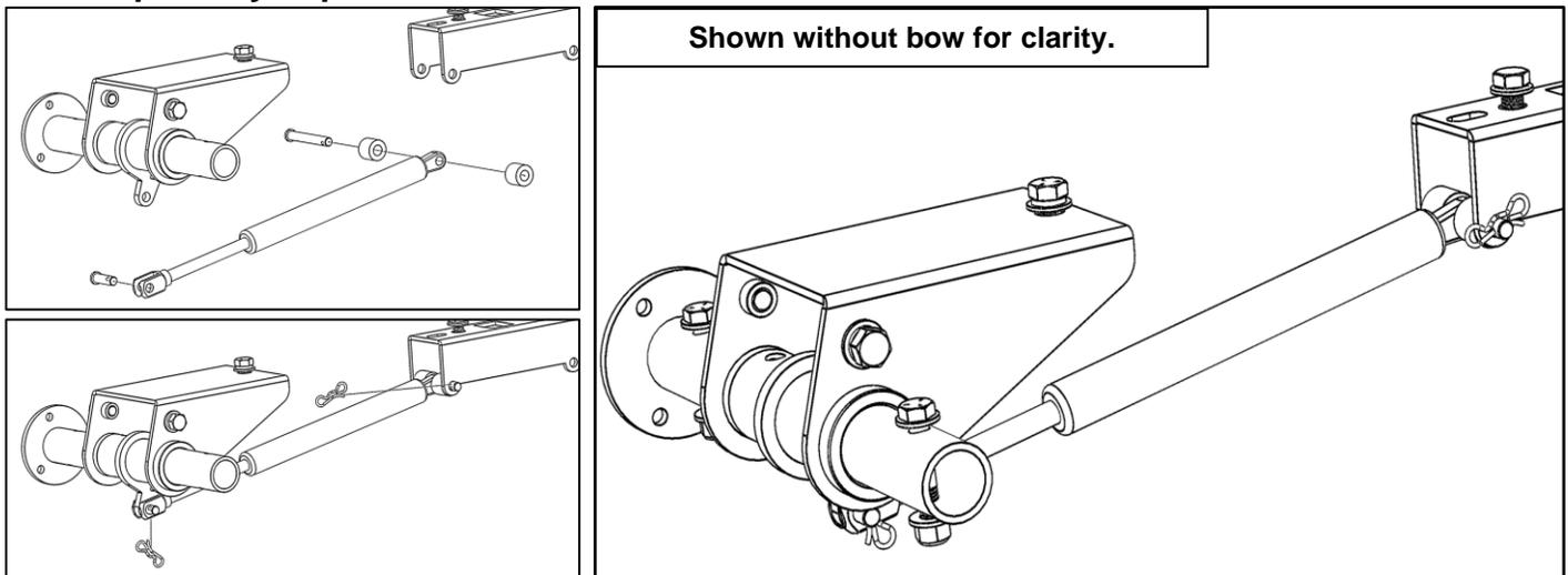
**Note:** In some situations, it may be easier to wait until handle assembly is installed to attach both ends of the damper. This is so you can use the handle to help shorten the distance between the two ends the damper.
