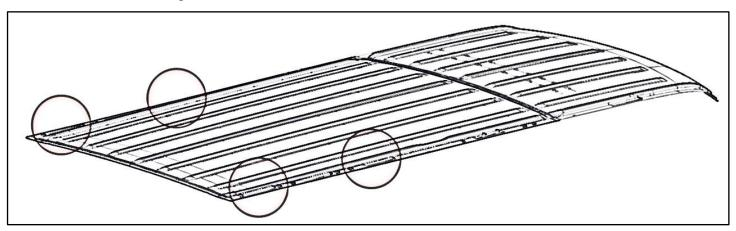
• Slide U-nut over the mounts in the locations shown. In the forward most of the two locations, only install one U-nut.
