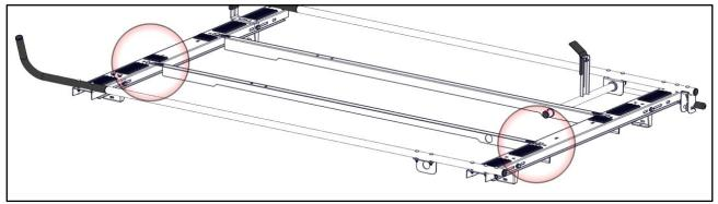
• Insert plastic bushings into the hanger bracket installed in Step 3 and the L-bracket, with flanges toward each other and to the inside, as shown. **Be sure to install the bushings in an orientation so they CANNOT fall out.**
