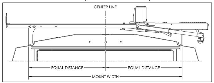
• Ensure the rear of the rack is far enough off the rear of the vehicle that when placing a ladder on the rack, the ladder does not hit the vehicle.
