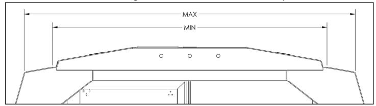
• Determine the best mounting width. Locate the corresponding slots on the ladder rack bow. Be sure to use the same slot at each ends of the ladder rack bow.
