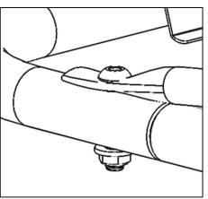
jam nut, bolt through front side channel and front crossbar.
