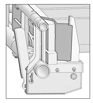
If ladder is thicker or the ladder hook is not clamping properly, adjust the ladder hook by removing flanged lock nuts on rear of ladder hook and then repositioning ladder hook to fit the ladder thickness.
