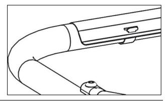
• Using #10 x 3/4" screws and #10 washers, bolt through top of wind deflector into press-in nuts on wind deflector straps.
