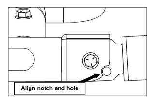
Insert the pin in the hole and lock the pin in the lock position.
