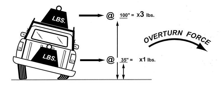
WEIGHT CARRIED ABOVE THE FLOOR OF THE TRUCK BED (E.G. ON AN OVERHEAD TRUCK RACK) WILL SIGNIFICANTLY INCREASE THE VEHICLE'S TENDENCY TO OVERTURN. ALWAYS KEEP HEAVY LOADS EVENLY DISTRIBUTED AND AS LOW AS POSSIBLE. IT IS IMPORTANT TO NOTE THAT THE KARGO MASTER RACK LOAD BEARING CAPACITY MAY BE GREATER THAN YOUR TRUCK'S GAWR OR GVWR CAPACITY, AND IS PROBABLY GREATER THAN THE WEIGHT THAT CAN BE SAFELY CARRIED OVERHEAD. RETIGHTEN ALL BOLTS AFTER FIRST USE, PERIODICALLY CHECK BOLTS FOR TIGHTNESS.
